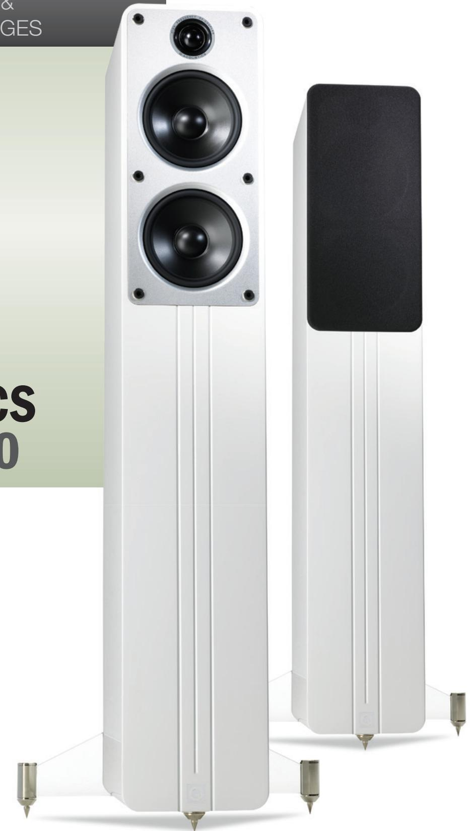
So despite its size, orientation and driver layout, the Concept 40 is a two-way design, using two identical drivers to deliver both bass and midrange, and leaving the highs to a single 25mm dome tweeter. Externally the driver is identical to the one used on the Concept 20, with a diameter of 125mm and a cone material of paper pulp covered by a thin coating of a material that Q Acoustics says is made from carbon-fibre and ceramic.
