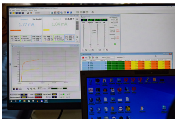
...and measured precisely by program. This allows the tubes to be selected in pairs...
