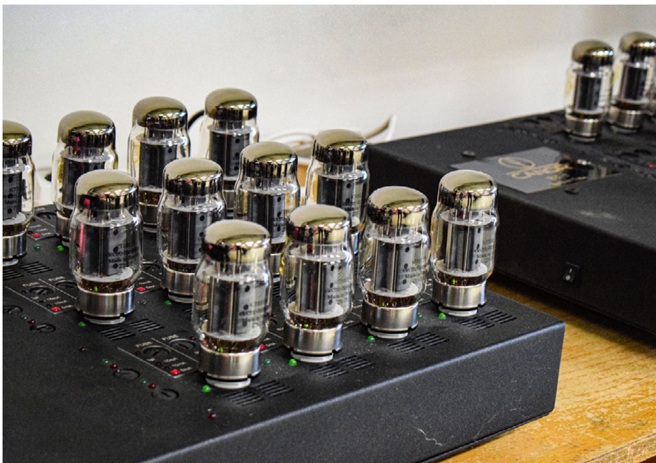
Before the measurement run, all tubes are baked for at least 200 hours
