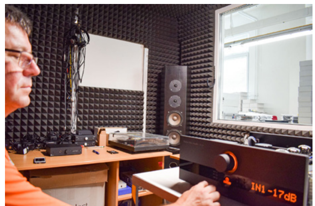
An employee checks every function of every device (and at a low noise level) in a sound-proofed room
