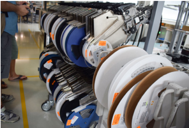
Inside the coils are tapes with thousands and thousands of miniaturized components: ICs, chips, etc ...
