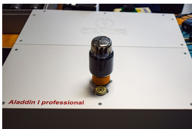
Afterwards, each tube is put into the Aladdin-1 measuring system ...
