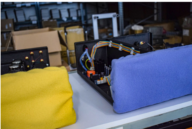
Precaution: when components are carried from one station to the next, they get solid coatings - against scratches
