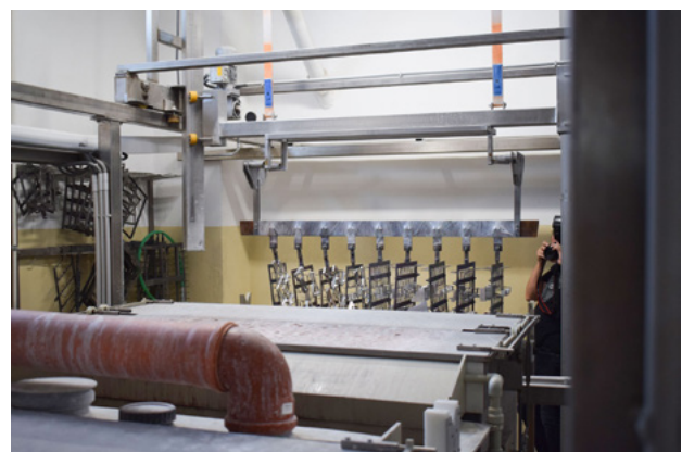
With the help of a sensor-controlled crane, the individual batches are ...
