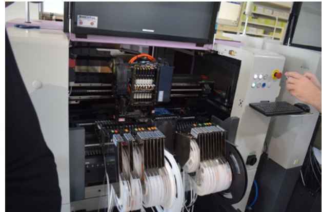
The super-fast pick-and-place machine places the components precisely in the right place
