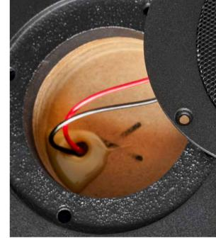
The tweeter uses an aluminum-ceramic dome tweeter, and, at 28 mm, it is slightly larger than normal. The flat driver sits in its own volume, which can hardly be called that: apart from the driver, not much else fits into the shell.
