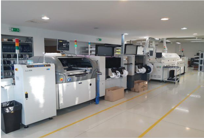
With the automated SMT production line, PCBs can be assembled in perfect quality and verlöten.
