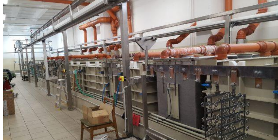
Aluminium parts are anodised in-house.
