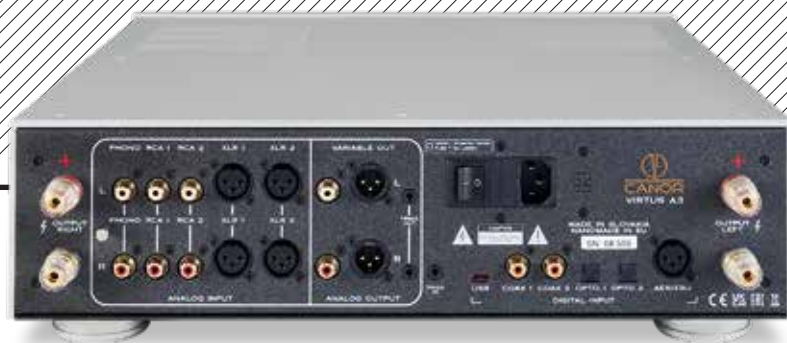
ABOVE: Single 4mm speaker binding posts and variable preamp outputs, on RCAs and XLRs, are joined by MM/MC phono and four line inputs (two balanced on XLR). Digital inputs include two optical, two coaxial, USB-C and AES/EBU
