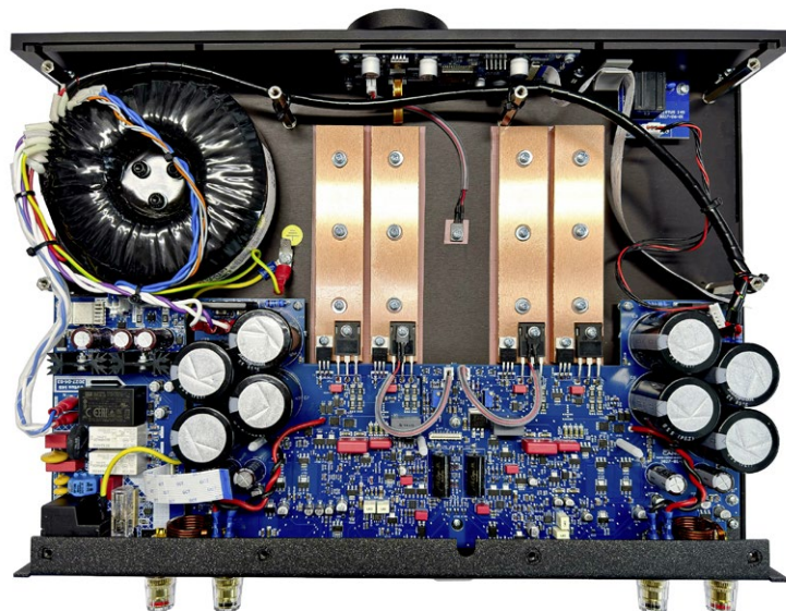
The silently operating fan and the copper heat sinks ensure a uniform temperature environment for the transistors.
