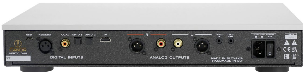
The rear of the DAC includes everything you could want digitally with USB, HDMI, coax, 2 x optical, and AES/EBU. Analog output is via fixed-level RCA and XLR outputs.
