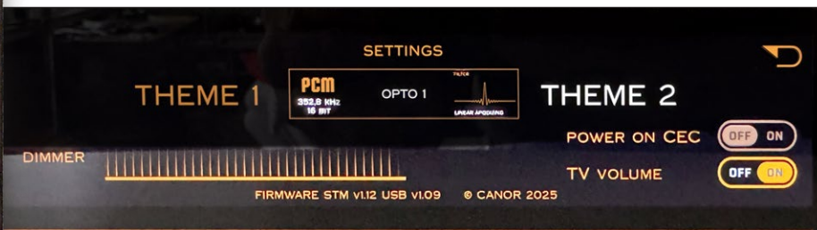
The color-switchable display provides comprehensive info on everything worth knowing if desired. At the push of a button, however, it only shows the most important items: input and filter.
